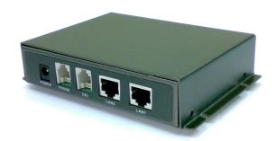
V102 is a VDSL LAN Extender providing a broadband transmission up to 100/60Mbps for downstream/upstream over single pair copper line or coaxial cable for point-to-point Ethernet connectivity. With 100/60Mbps data rate, V102 Series supports transmission distance up to 300 meters and 30/10 Mbps for 1km long range connection. Users may also select a fixed data rate or a fixed SNR margin for different copper line ranging.
