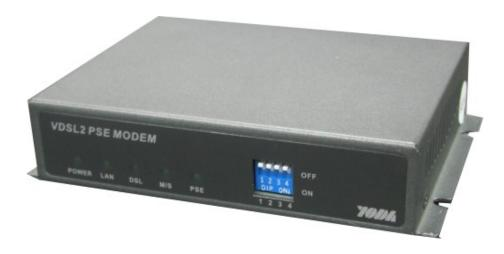
V102M-PSE is a VDSL2 LAN Extender providing a broadband transmission up to 100/100Mbps for downstream/upstream over single pair copper line or coaxial cable for point-to-point Ethernet connectivity. With 100/100Mbps data rate, V102M-PSE supports transmission distance up to 250 meters and less data rate for 1.5km long range connection. Users may also select a fixed data rate or a fixed SNR margin for different copper line ranging.
