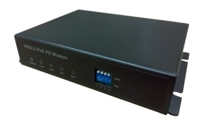
V102M-PD is a VDSL2 LAN Extender providing a broadband transmission up to 100/100Mbps for downstream/upstream over single pair copper line for point-to-point Ethernet connectivity. With 100/100Mbps data rate, V102M-PD supports transmission distance up to 250 meters and less data rate for 1.5km long range connection. Users may also select a fixed data rate or a fixed SNR margin for different copper line ranging.
