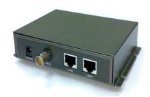
V102M-BNC is a Coax LAN Extender providing a broadband transmission up to 100/100Mbps for downstream/upstream over coaxial cable for point-to-point Ethernet connectivity. With 100/100Mbps data rate, V102M-BNC supports transmission distance up to 700 meters and less data rate for 3km long range connection. Users may also select a fixed data rate or a fixed SNR margin for different copper line ranging.
