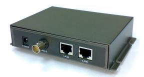
V102-BNC is a Cable LAN Extender providing a broadband transmission up to 100/60Mbps for downstream/upstream over coaxial cable for point-to-point Ethernet connectivity. With 100/60Mbps data rate, V102 Series supports transmission distance up to 300 meters and 30/10 Mbps for 1km long range connection. Users may also select a fixed data rate or a fixed SNR margin for different coaxial cable ranging.
