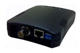
V101 Series is a VDSL LAN Extender providing a broadband transmission up to 100/60Mbps for downstream/upstream over single pair copper line or coaxial cable for point-to-point Ethernet connectivity. With 100/60Mbps data rate, V101 Series supports transmission distance up to 300 meters and 30/10 Mbps for 1km long range connection. Users may also select a fixed data rate or a fixed SNR margin for different copper line ranging.
