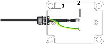
6. The other end is also <u>connected to the RJ45 connector</u> (1), and <u>make the nut locked</u> (2) into the waterproof set.
