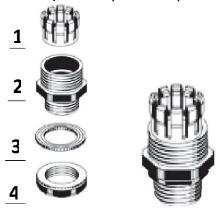
3. The pre-assembled network and grounding cables to pass through the waterproof cover set as shown.
