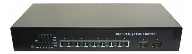
PS820G series, a 10-port Gigabit PoE+ Switch, is a standard Gigabit Ethernet switch that meets all IEEE 802.3/u/x/z/ab/af/at standards. The switch includes 8-Port 10/100/1000Mbps RJ-45 with PoE+ function and 2-Port Gigabit SFP for Fiber. It is an ideal solution for applications of wireless AP, IP phones and IP cameras.
