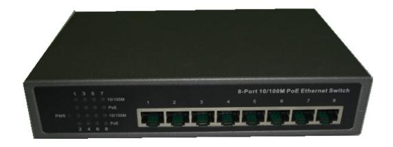
The PS800E is a 8-port Fast Ethernet, IEEE 802.3at/af PoE Switch utilizing a compact form factor with per PoE power of 15.4w or 30w and total power budget of 120w.
