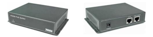
PS300 is a high power PoE Splitter for use in Power over Ethernet systems. With Ethernet Input (data + power) port and Output (data only) port, PS300 may split power from existing LAN cable and convert up to 12VDC/2A for power hungry applications such as Wireless APs, Security cameras and IP Phones. The internal current limit, short-circuit and overload protection are implemented to provide up to 12VDC/2A for use of DC output power.
