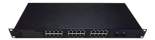
Yoda PS2420GT series provides 24 Gigabit Ethernet Switch ports with IEEE 802.3at/af PoE interfaces and 2 10G SFP/SFP+ open slots. It supports MDI / MDI-X convertible on 24-10/100/1000Mbps ports and provides PoE injecting function on PoE ports which are IEEE 802.3af/at compliant.
