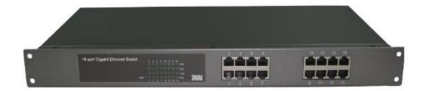
The PS1600G series features a 16-ports 10/100/1000Mbps Gigabit Ethernet Switch with IEEE 802.3at/af Power over Ethernet interfaces. It supports MDI/MDI-X function on all 10/100/1000Mbps ports and provides Power injection on each LAN port which complies to IEEE 802.3af (15W) and 802.3at (30W) PoE powered devices.
