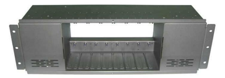
The PPS800, an 8-bay 19" power chassis, is designed specifically to station for high power PoE Injectors with input 100-240VAC and output 24VDC. With plug & play features for easy installation, each bay of PPS800 can be plugged in for one high power PoE injector such as PI300 to supply high power for remote applications.
