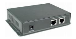
PI300 is a high power, PSE Power Injector for use in Power over Ethernet systems. With Ethernet Input (data only) port and Output (data + power) port, PI300 may deliver up to 60 Watts over existing LAN cable to power up PoE PD devices for power hungry PoE applications such as Wireless APs, Security cameras and IP Phones. The internal current limit, short-circuit and overload protection are implemented to provide up to 60W of PSE output power.
