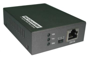
PC300G is a Gigabit Power-over-Ethernet (PoE) Converter providing a 10/100/1000Mbps Ethernet transmission for overall 100-meter distance and via its 12/19/24V DIP Switch to flexibly select PoE power out of 12/19/24V for passive PoE networking devices such as wifi AP.
