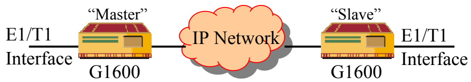
Figure 1. E1/T1 Leased Line Connection over IP Network
